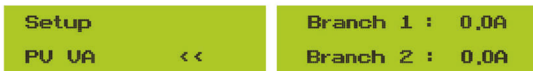
Pic 8.16 PV String current
