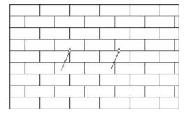
Insert the expansion tubes into the holes and tighten them. Install the bracket with the expansion screws.
