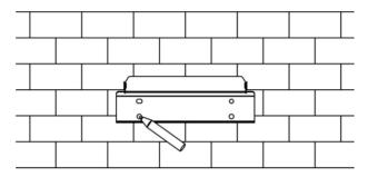
Drill holes with electric drill, make sure the holes are at least 50mm deep, and then tighten the expansion tubes.
