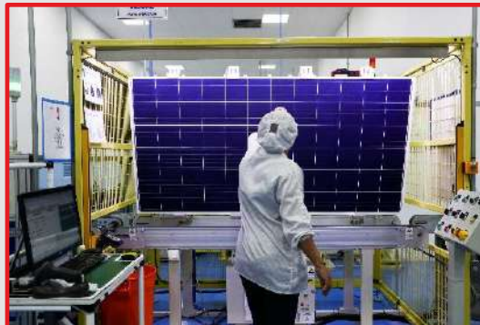
Final Visual Inspection
